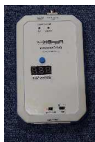
Fig. 11. Prototype system of the PWoF power supply module.
